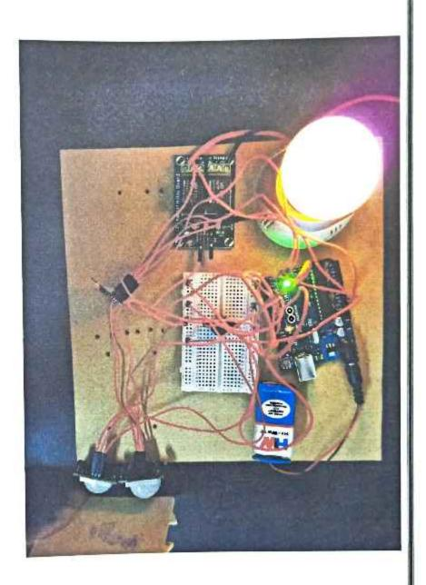
In the above picture the Arduino UNO board is connected to breadboard, 2 channel relay board, two PIR sensors and ESP8266 using male to male and male to female jumper wires. 2 channel relay board connects Arduino UNO board to the bulb. The buzzer is placed on the breadboard to make sound when an object passes through the PIR sensors.
