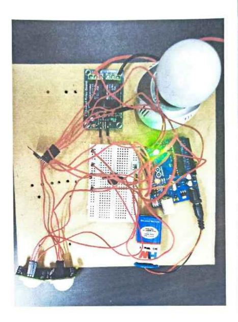
In the above picture the Arduino UNO board is connected to breadboard, 2channel relay board, two PIR sensors and ESP8266 using male to male and male to female jumper wires. 2-channel relay board connects Arduino UNO board to the bulb.
